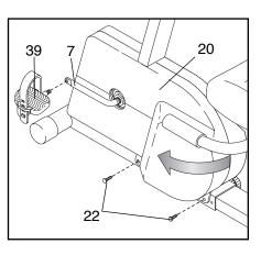
Using an adjustable wrench, turn the Left Pedal (39) clockwise and remove it. Next, remove the indicated #8 x 1/4" Screws (22). Grasp both Side Shields and gently pull them apart. Turn the left arm of the Crank (7) to the position shown, and then carefully slide the Left Side Shield forward and remove it.
